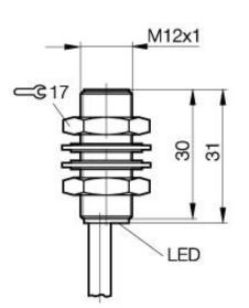
**Inductive Sensors** BES 516-370-E4-Y-PU M12x1 x 33 normally-closed Sn=2mm shielded
